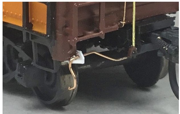
Styrene uncoupling lever bracket with uncoupling lever installed.
