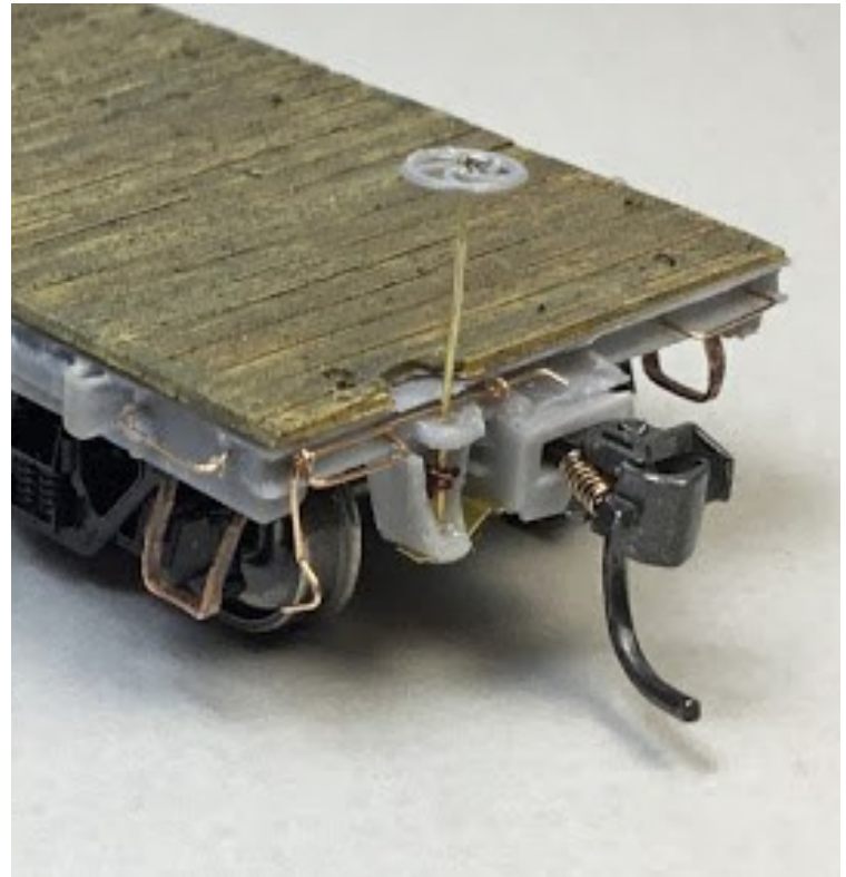
Flat car with Type B, top mounted coupler with eye bolt brackets.
