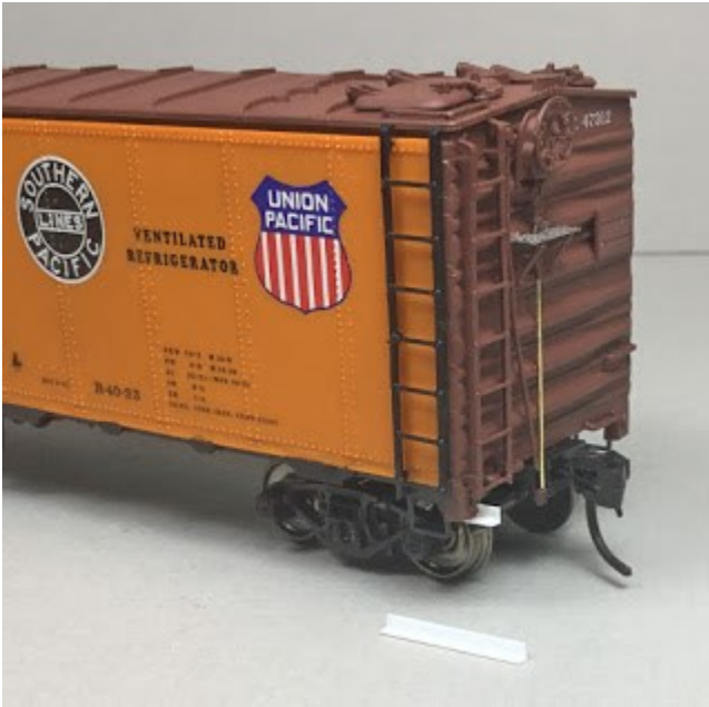
Side view of Evergreen .060" angle installed.
