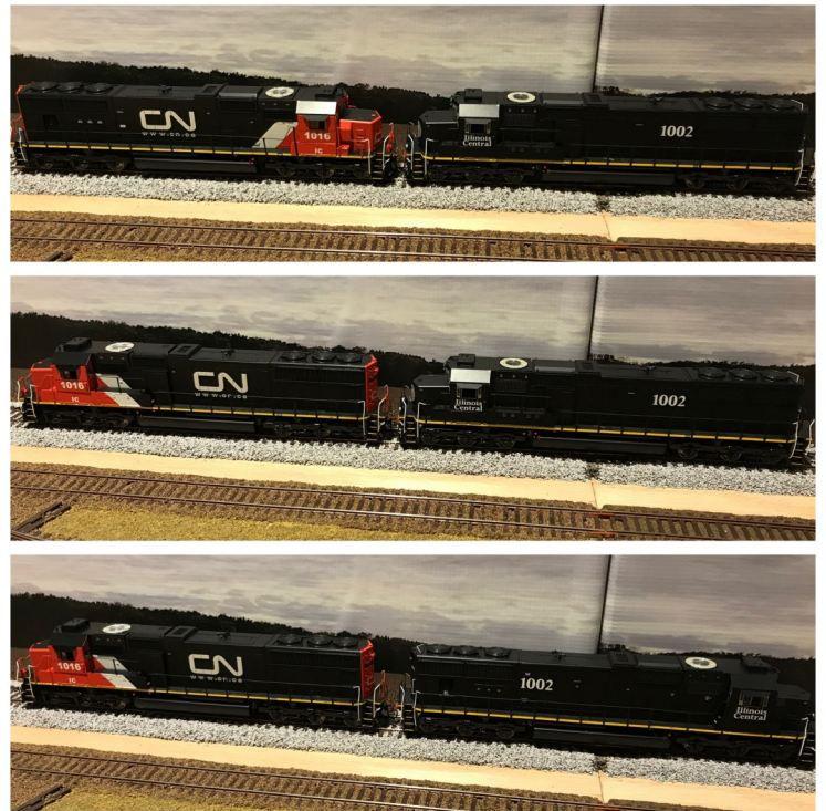
Image 1- The variable positions of engines for consisting: Top, Head to Head, Middle, Head to Tail, Bottom, Tail to Tail
