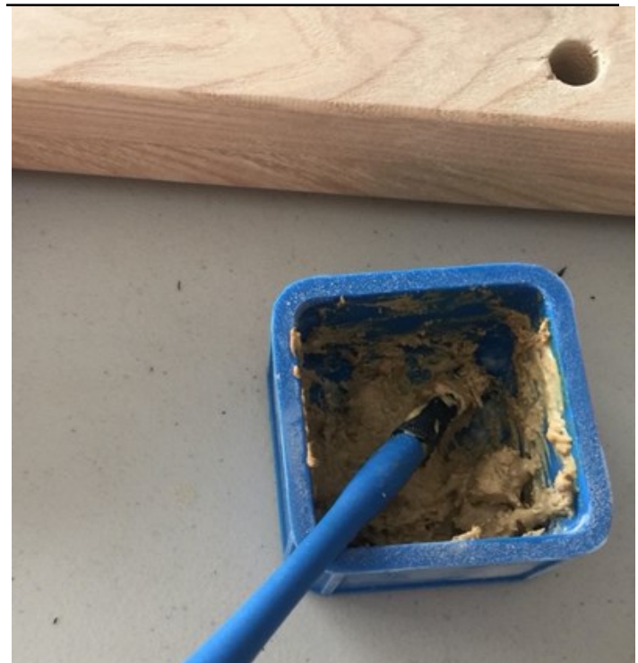
Figure 2. Silicon tub and mixing tool depicting filler mixed with wood glue
