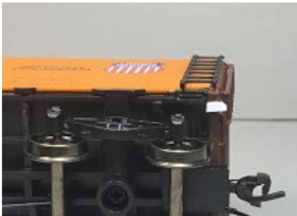
Bottom view of Evergreen .060" angle installed.
