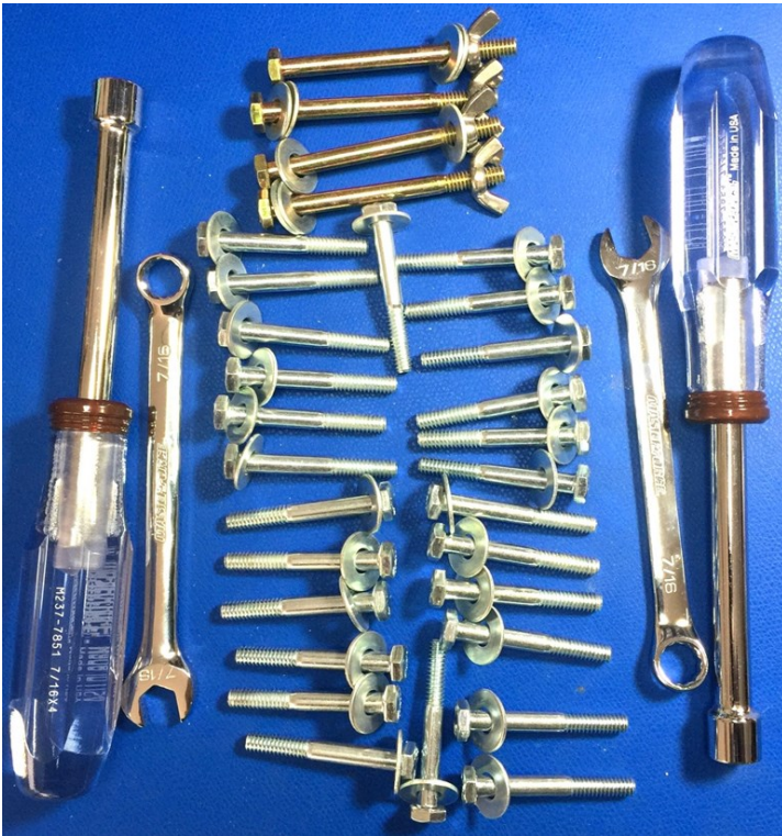
Figure 7: Hardware and tools required to assemble each photography stand
