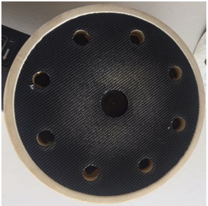
Figure 5. Bottom of sander showing the “hooks” used to attach the pads to the sander (Note: the larger holes are where sawdust exists the sander into an attached vacuum)
