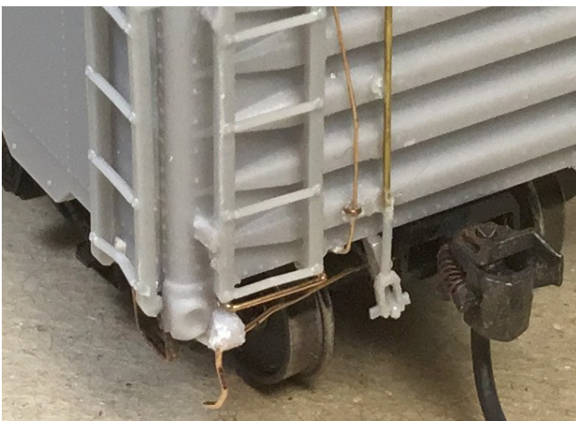
Uncoupling lever bracket is photo-etched one from Yarmouth Models.
