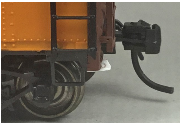
Number 78 hole drilled in shaped uncoupling lever bracket.
