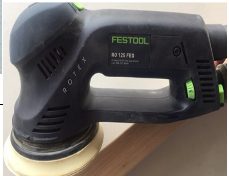
Figure 4. Festool Rotex RO 125 FEQ sander used to prepare photography stand boards for finishing (Note: The green button in the top left of this photograph is the on-off switch)
