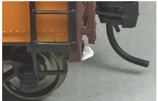
Installed angle shaped with PBL #803 Gate nippers.
