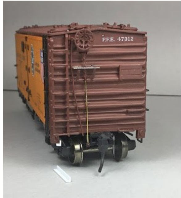
Front view of Evergreen .060" angle installed.
