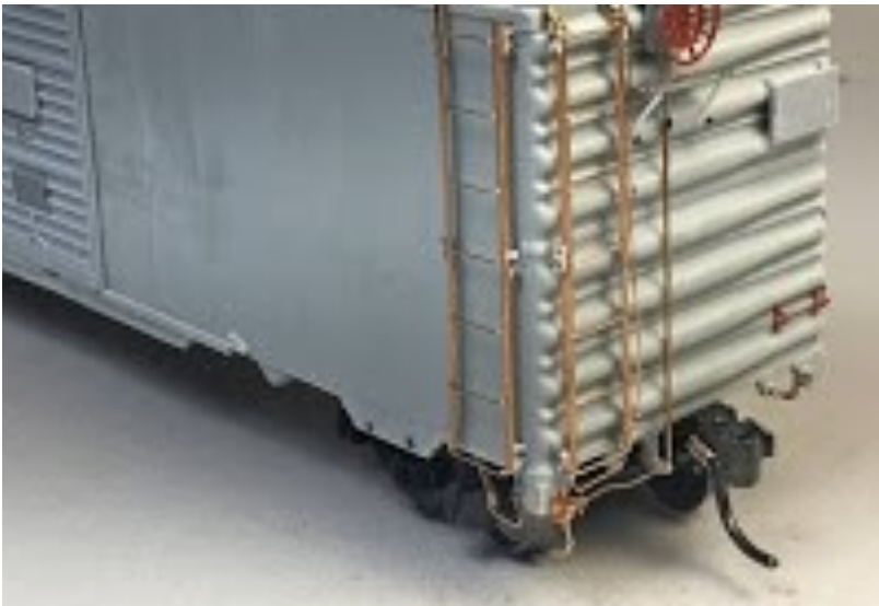
Uncoupling lever bracket is photo-etched one from Yarmouth Models.
