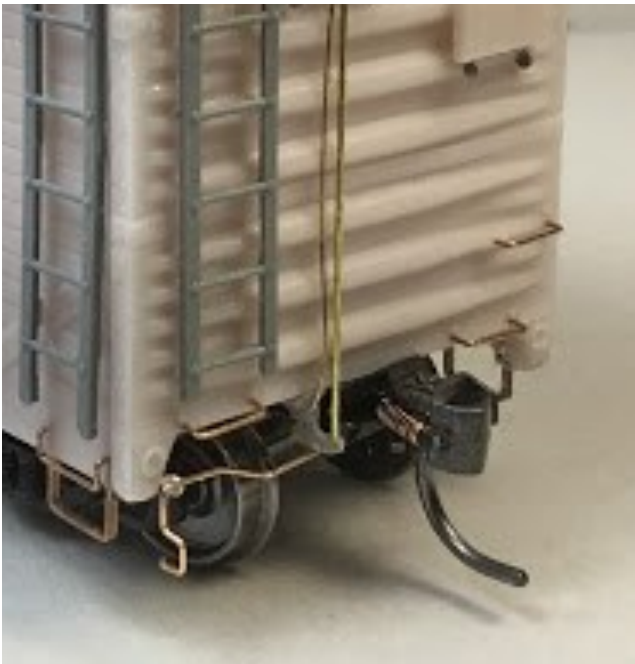
Box car with Type E bottom operated coupler with eye bolt brackets.
