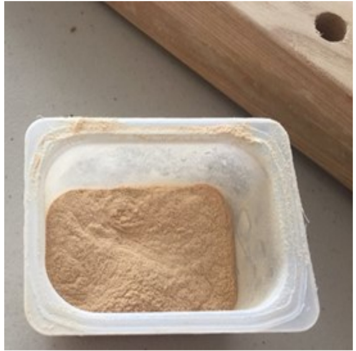
Figure 1. Ash wood powder used to repair woodworking defects
