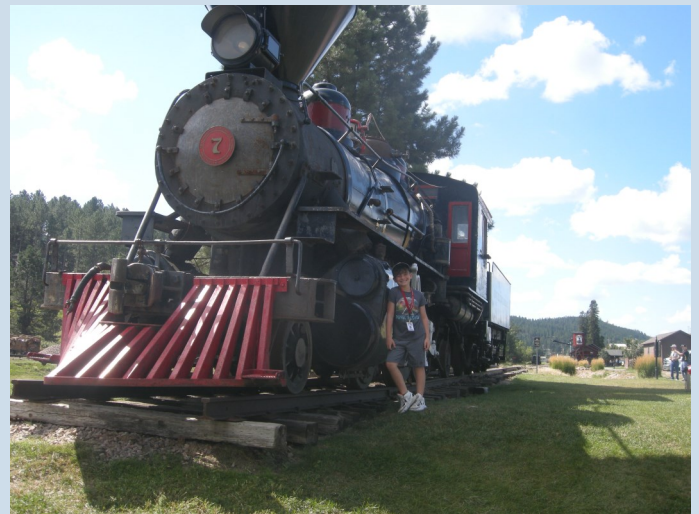
Finnlay strikes a pose next to Number 7. Black Hills Central Railroad Engine #7 is a 2-6-2 with tender built by Baldwin Locomotive Works for the Ozan-Graysonia Lumber Company in 1919.
