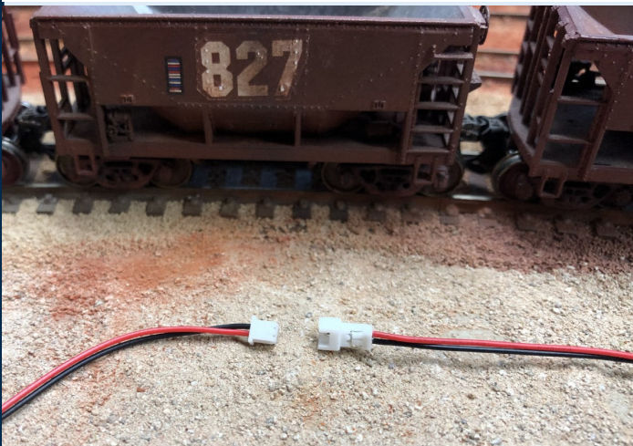
The Micro JST connector allows quick removal of the speaker.
