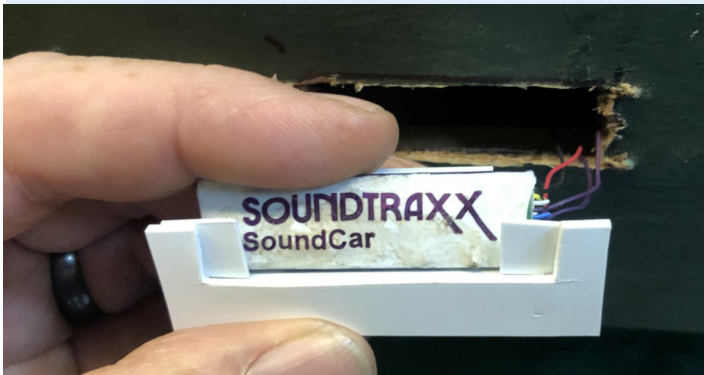
The Soundtraxx decoder, already in it's holder. Note the four wires to the tight, and the fascia cutout.
