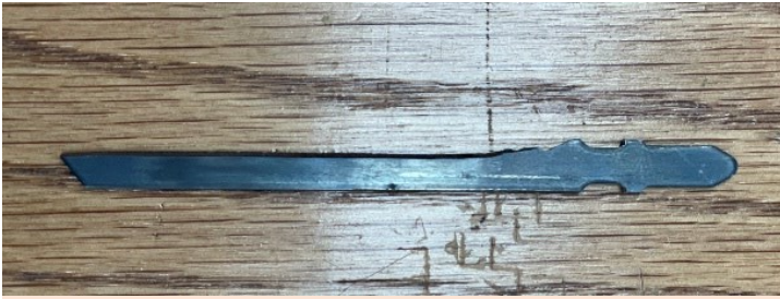
File teeth off jig saw blade to cut the foam easily
