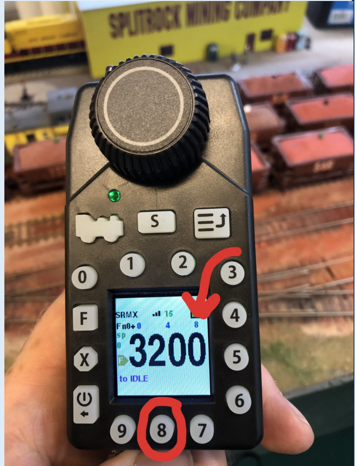
Pushing Function 8 four times activates the card. The soundcard must be connected to track power to get the DCC signal.
