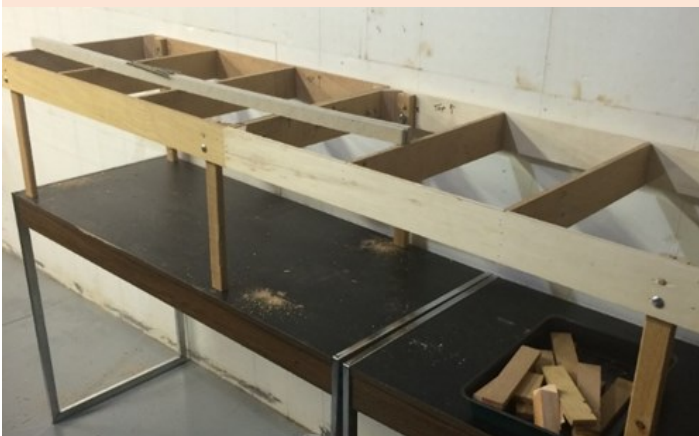
Module constructed using ripped down plywood vs dimensional lumber
