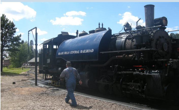
Black Hills Central No. 110 is a 2-6-6-2T (Tank) articulated mallet steam locomotive built by Baldwin in 1928 for Weyerhaeuser Timber Co.
