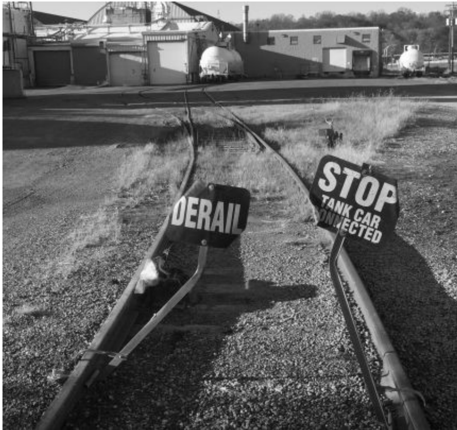
Photo 1- The blue "flags" indicate the track is protected by a derail and that the tank car in the background is connected to the building. The blue flags are protecting the two tracks behind the turnout.
