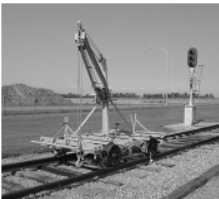
The newest piece of equipment on display at the club and waiting to be refurbished is this Fairmont Motors track derrick.
