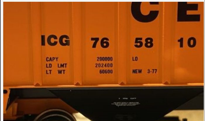
Image 6: Using the loaded and unloaded weights, the scale is programmed to display the weight for the car.
