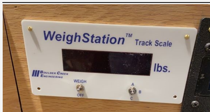
Image 4: Switch on the left is On/Off, and the right switch is for choosing the operating mode (A,B or C).
