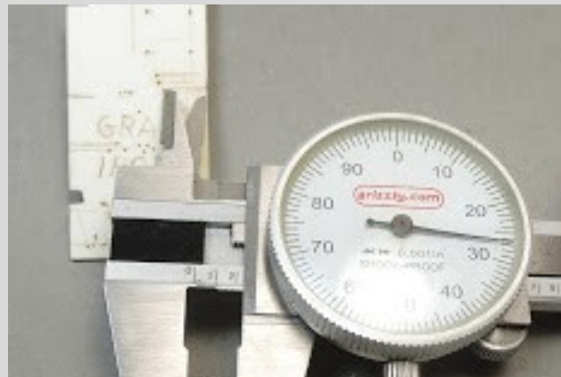
Caliper used to mark hole for drilling
