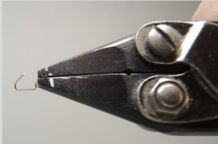
Finished drop grab iron
