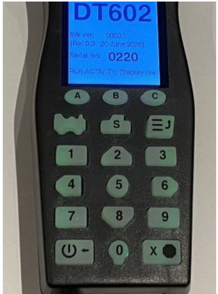
Image 4: Pushing the locomotive shaped button beneath button A allows you to enter your Loco address. Below button B is the turnout button ("S"), below button C is the Menu button, and you exit menus by pushing the X (stop sign) button in the lower right.
