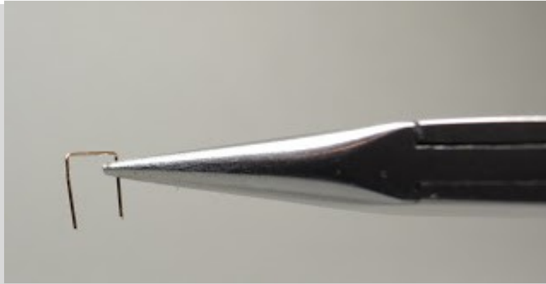
Finished straight grab iron
