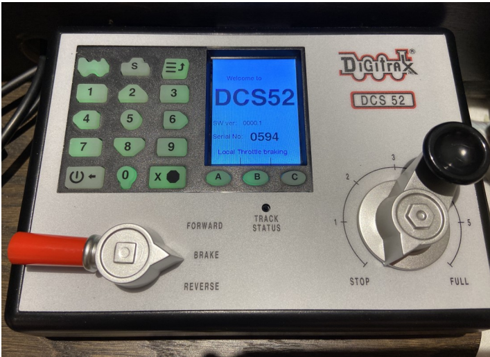
Image 2: Digitrax DCS 52 Command Station.
