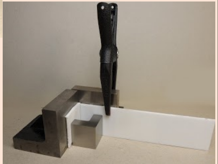
Machinist blocks used to create an "L" shaped section of wall.
