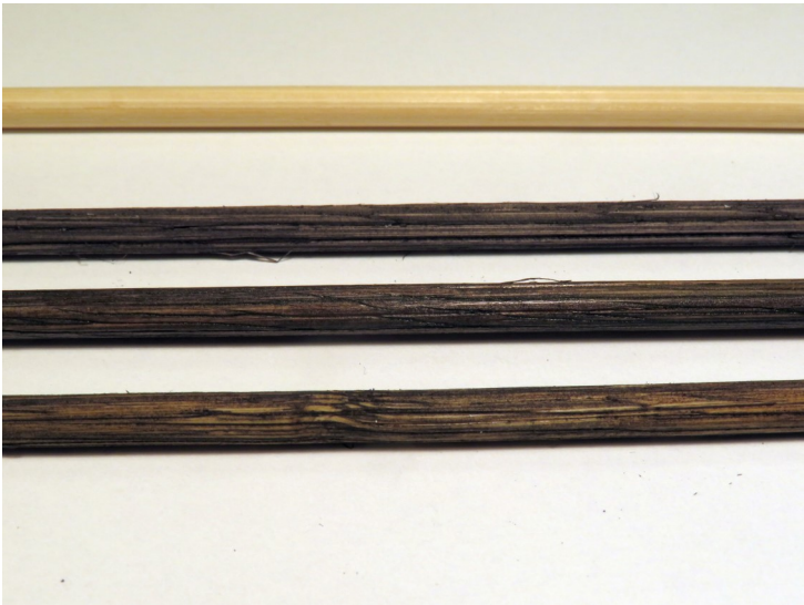
From top to bottom– unmodified, Timberline creosote stain, mahogany oil stain, Timberline Driftwood followed by brown water color pen. The bottom three are textured.
